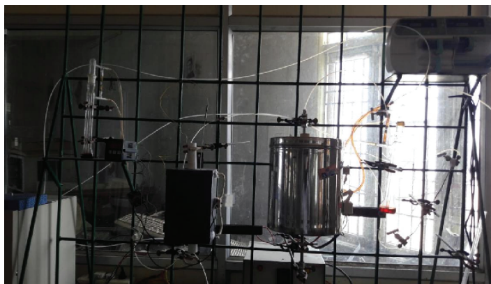
Fig. 3. Manual setup for CO 2 adsorption studies
